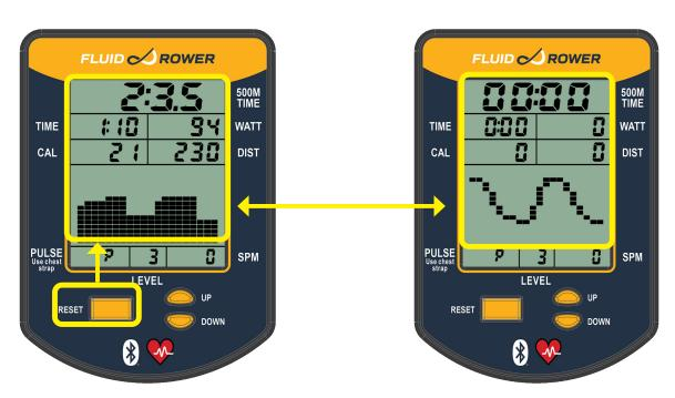
To clear workout data press and hold **RESET for 3+ seconds**.
